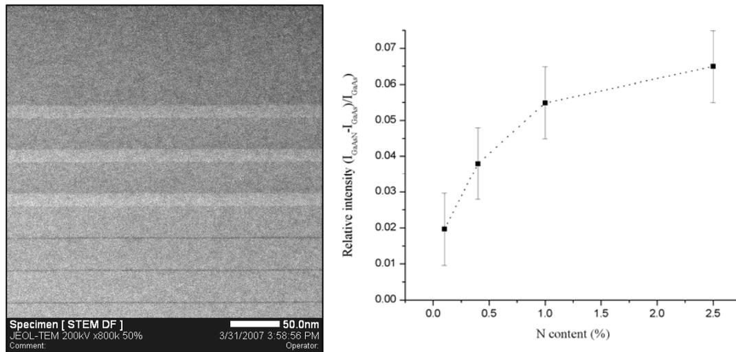
FIG. 1. (a) Low magnification HAADF-STEM images of the GaAsN quantum wells with 2.5%N. (b) Plot of the evolution of contrast with N content from a series of GaAsN Quantum wells.
