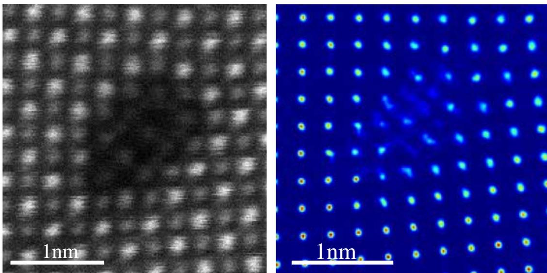
FIG. 2. (a) Representative Z-contrast image of a dislocation core in a low-angle SrTiO<sub>3</sub> grain boundary. (b) Probability distribution of atom locations based on images of ~200 cores.
