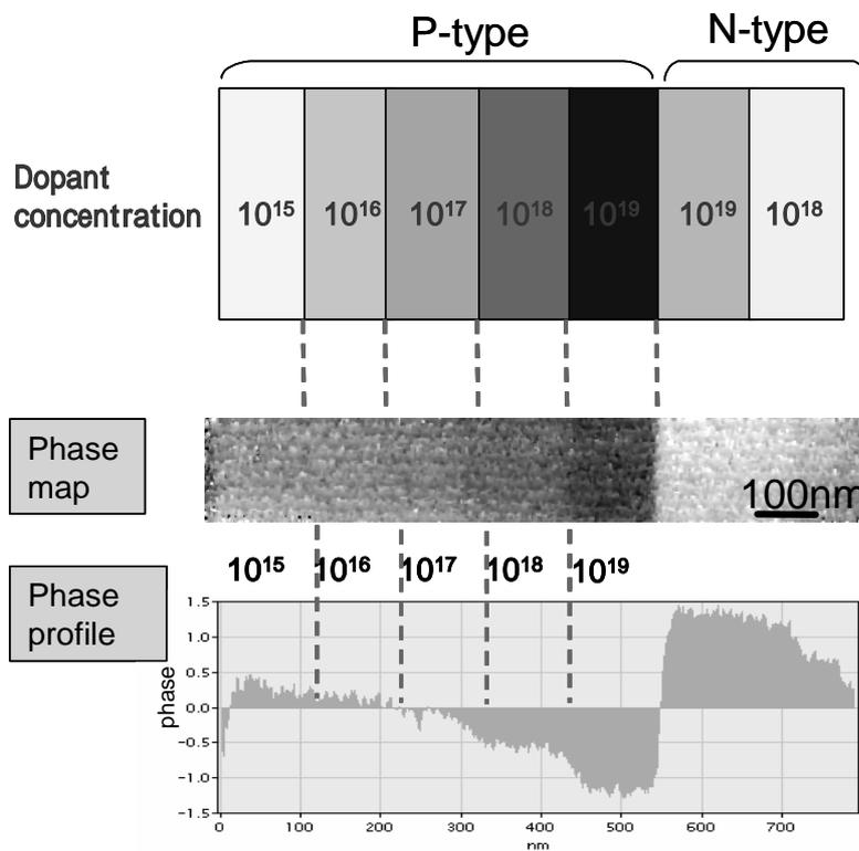
FIG. 2. Dopant profiling in GaAs by electron holography.
