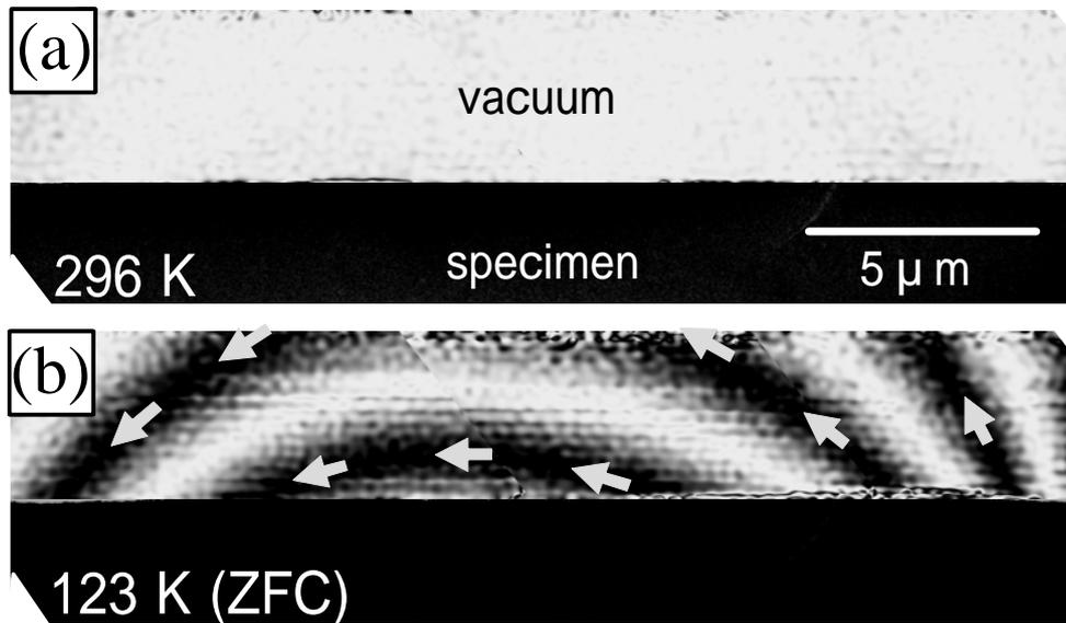
FIG. 1. Reconstructed interference micrograph of 250 nm thick random assembly of Co/CoO clusters at (a) room temperature and (b) 123 K.
