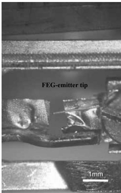
Fig.1 The developed specimen cassette and the fixed FEG-emitter tip.
