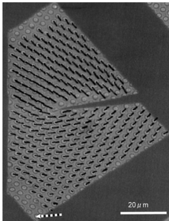
Fig.2 The shadow image distortion showing the field distribution.
