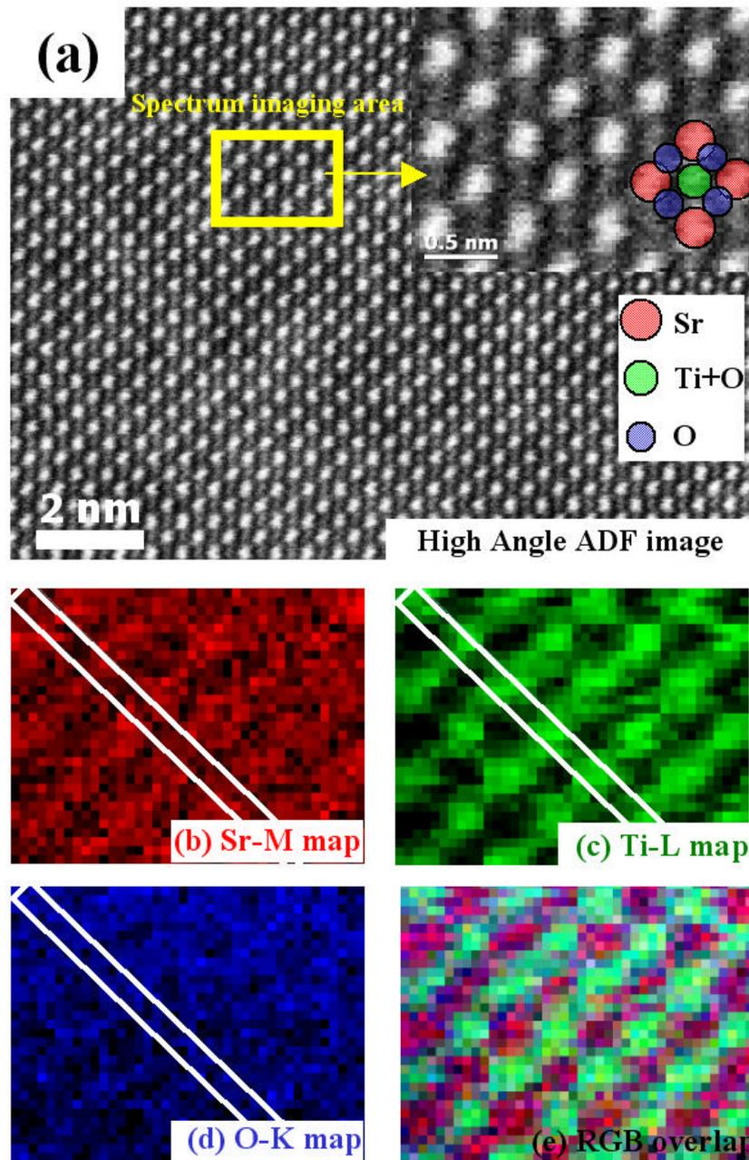
Fig 1. EELS elemental mapping with a spectrum imaging method.
