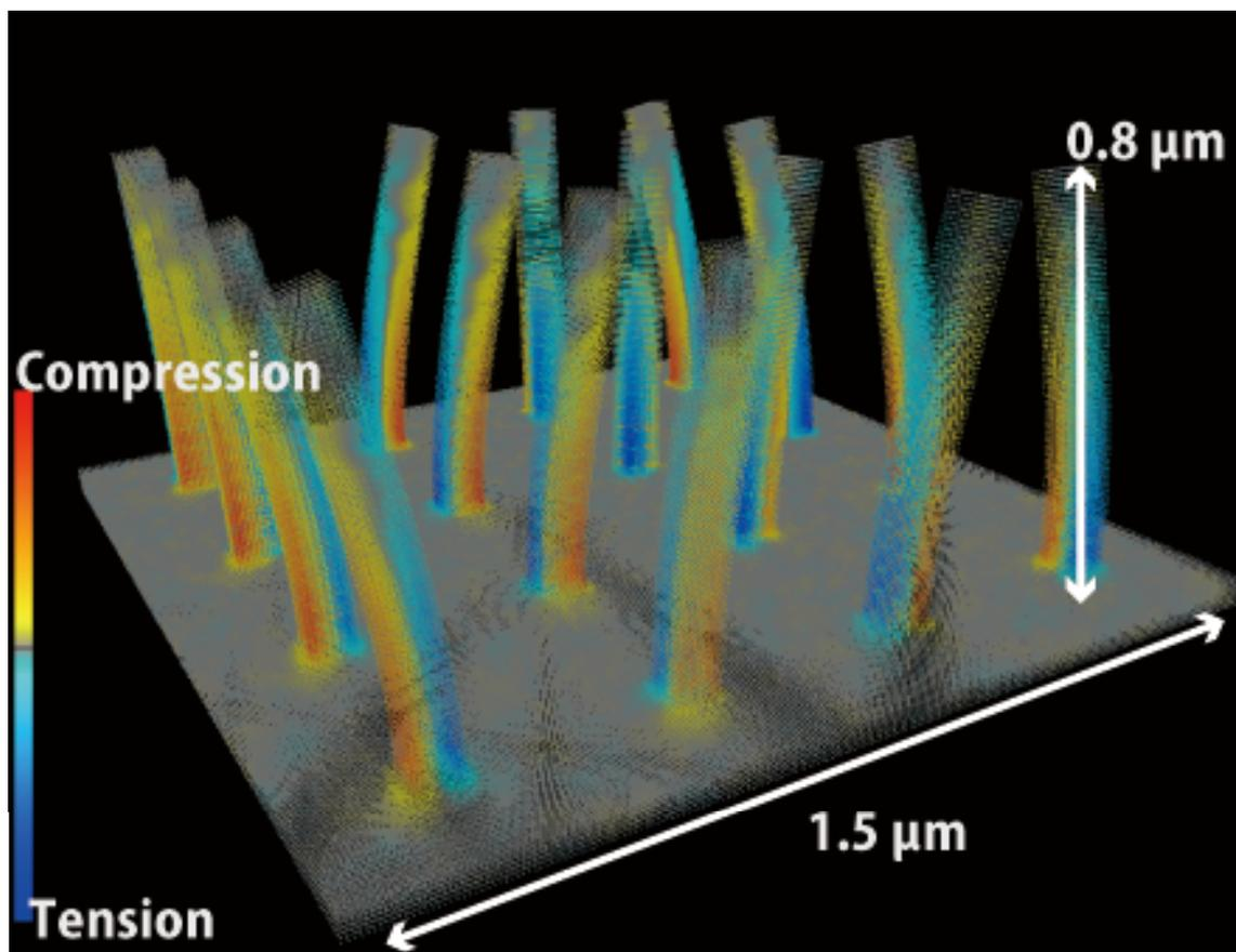
FIG. 2. A snapshot of the FCGP simulation of the oscillating nanorods. About 16,000 atoms are coarse-grained to one particle in this simulation.
