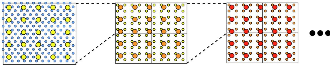
FIG. 1. Schematic illustration of the recursive coarse-graining method. At first we coarse-grain the atomic system (light-blue balls) to obtain the coarse-grained system (yellow balls). The coarse-grained system (yellow balls) is extended assuming the periodic boundary condition and the system is again coarse-grained. Continuing this procedure recursively, we can obtain massively coarse-grained system.
