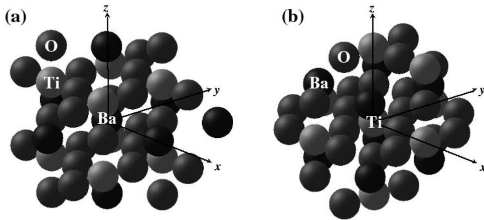
FIG. 1. The initial atomic structures of structural models for the BaTiO<sub>3</sub> ceramic nanoclusters (40 atoms) constructed from the cubic Perovskite BaTiO<sub>3</sub> crystal structure; (a) one of the Ba-centered model and (b) one of the Ti-centered model.
