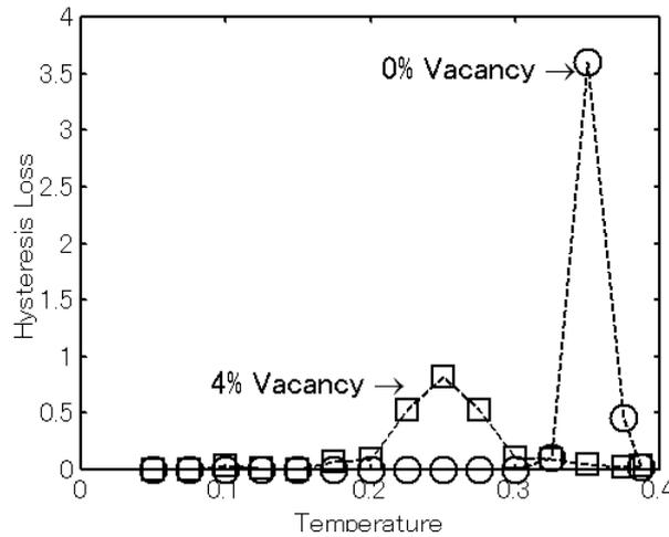
FIG.1 Temperature dependence of the damping capacity calculated by molecular dynamics as hysteresis loss for cyclic stress in the model crystals with and without vacancies as models for point lattice defects.---
