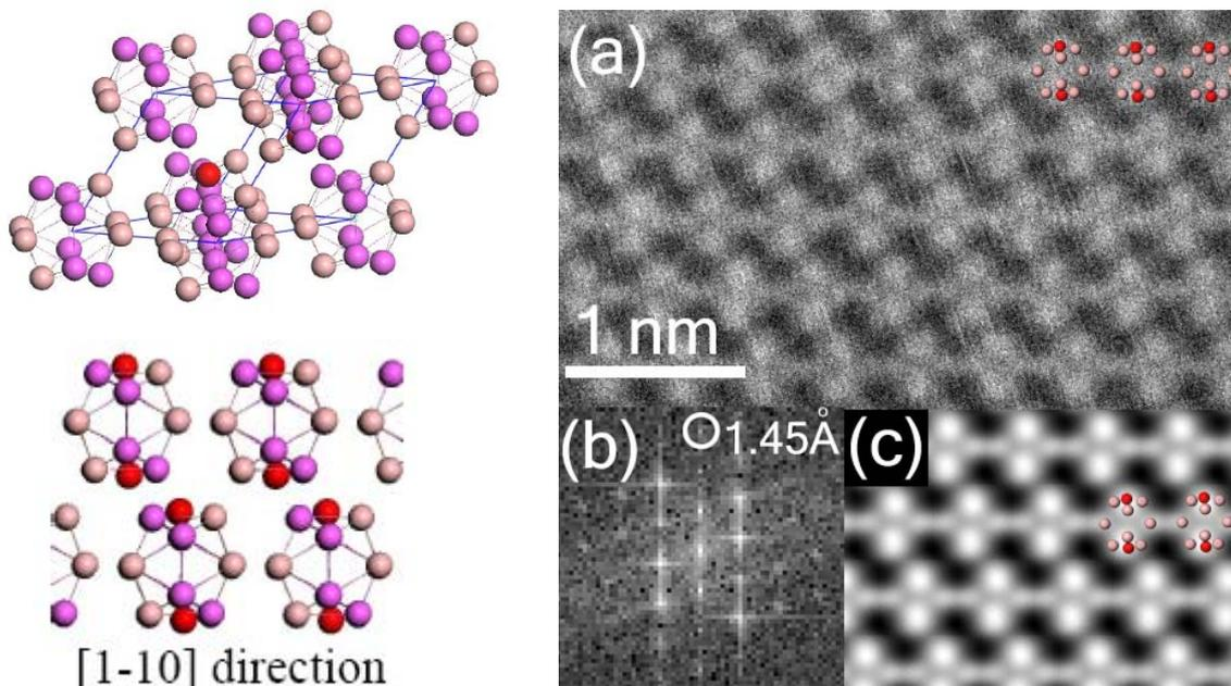
Fig. 1 The unit cell of the boron suboxide (top left) and the images of the boron cluster in [1-10] projection (bottom left). The right panel shows the experimental HAADF image of the boron suboxide also in [1-10] projection (a) with the corresponding power spectrum of the Fourier transform of the image (b) and the Fourier averaged reconstruction of the cluster image.
