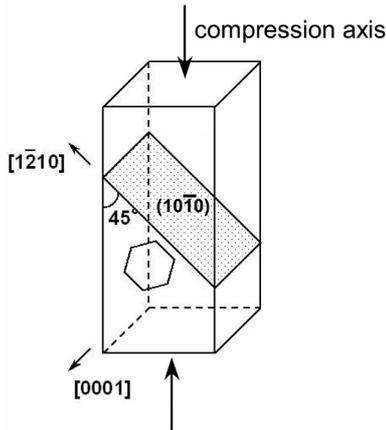
FIG. 1. Crystallographic orientation of the specimen for compression testing.
