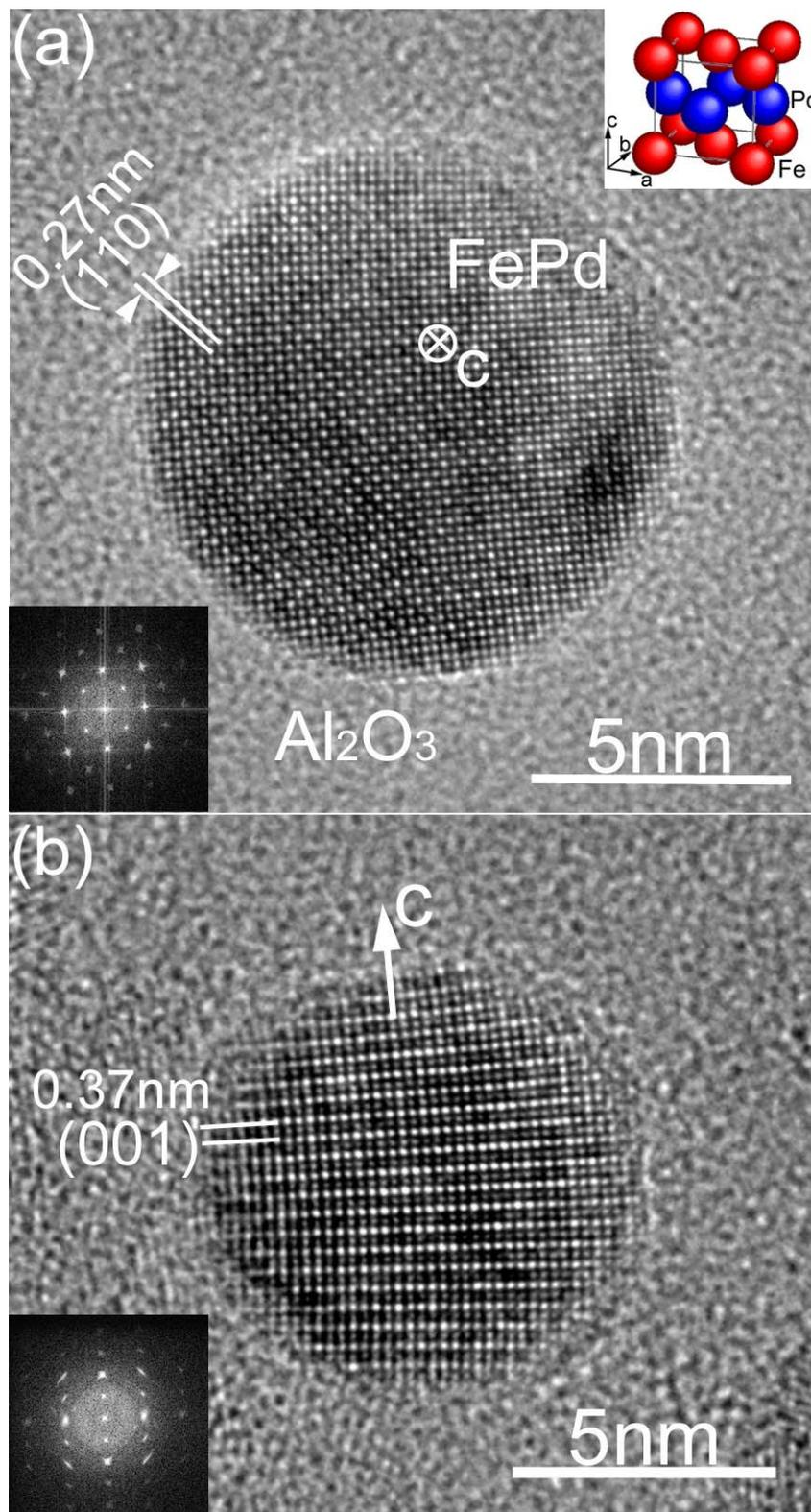
FIG 1. HREM images of FePd nanoparticles with the L<sub>10</sub> structure: (a) beam || [001], (b) beam || [100]. A schematic illustration of the L<sub>10</sub> structure is shown in the inset.
