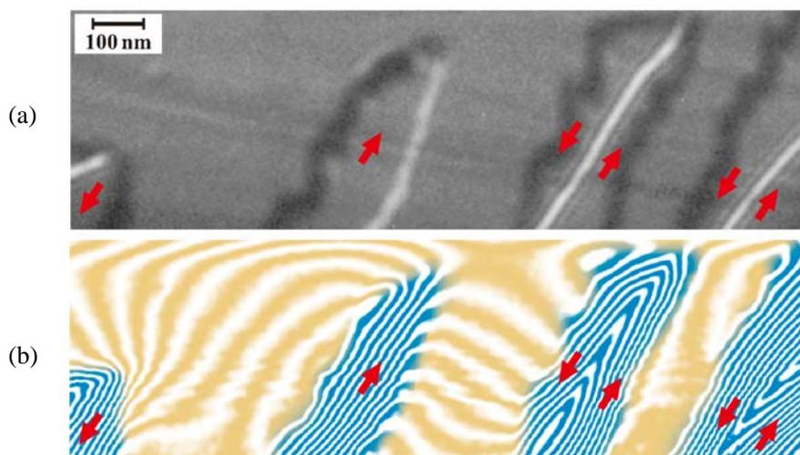
FIG. 2. Growth of ferromagnetic domains in colossal magnetoresistance manganite,  $\text{La}_{0.25}\text{Pr}_{0.375}\text{Ca}_{0.375}\text{MnO}_3$ , thin film at  $T = 62.4$  K: (a) Lorentz micrograph; (b) interference micrograph.
