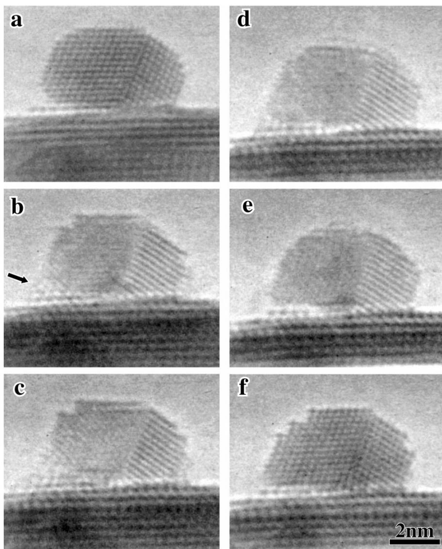
FIG. 1. Sequential TEM images of Pt particle on CeO<sub>2</sub> in the gases of 10<sup>-3</sup>Pa of CO+O<sub>2</sub>(a), O<sub>2</sub>(b), in vacuum, CO(d), CO+O<sub>2</sub>(e), O<sub>2</sub>(f).
