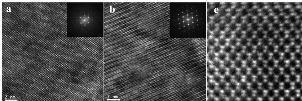
FIG. 2. High-resolution images of (110) diamond lattice after 30 keV FIB sample preparation (a); after using 5 keV FIB milling on final stage (b); magnified image of central area of previous image (c). Corresponding power spectrums are shown on inserts.
