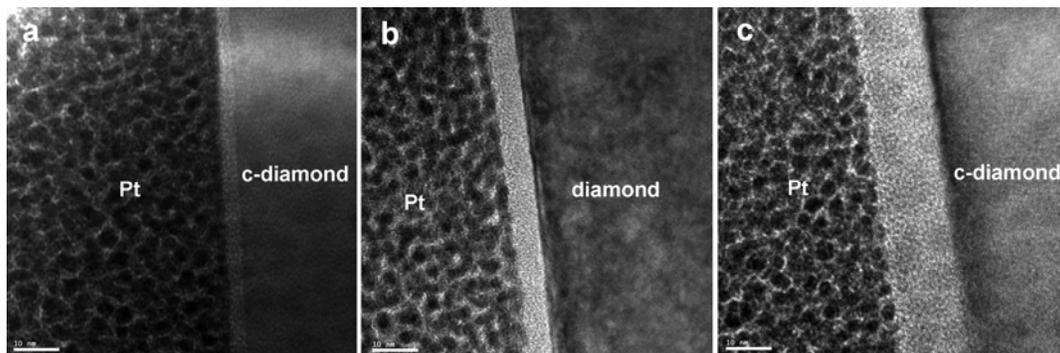
FIG. 1. Cross-sectional images of the side-wall (a-c) damage layers in the diamond samples after FIB milling with 5 (a), 10 (b) and 30 (c) keV  $\text{Ga}^+$  ions.
