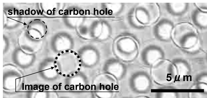
FIG. 1. Simultaneously recorded image and shadow image of Quantifoil 2/2
