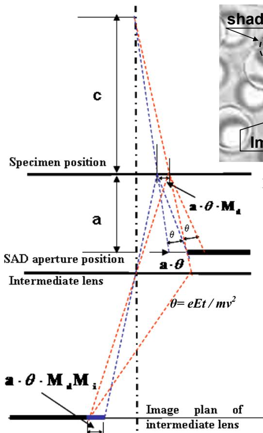
FIG. 2. The ray diagram of the electron optics of the SID method if the objective lens is turned off.
