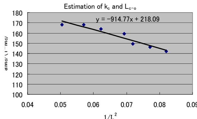
FIG. 3. Estimation of the distance between the condenser and the objective lens  $L_{c-o}$  and the lens constant of condenser lens  $k_c$
