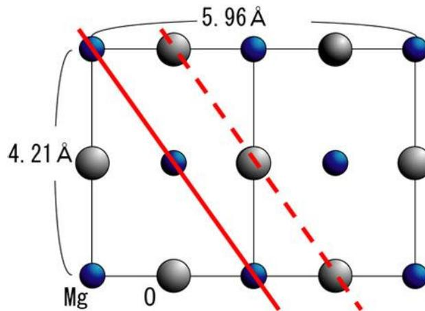
Fig. 1. Projected figure of MgO [110].
