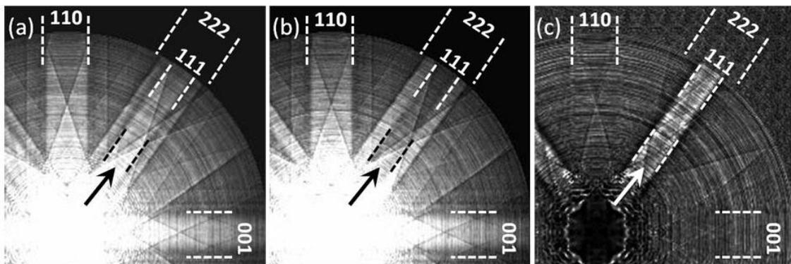
Fig. 2. Simulated diffraction images. 111 band is indicated by arrow. (a) Probe locate at Mg site, (b) Probe locate at O site, (c) The ratio pattern of (a) to (b).
