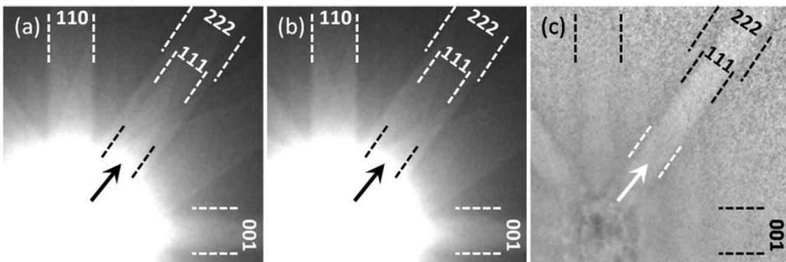
Fig. 3. Experimental diffraction images. 111 band is indicated by arrow. (a) Probe locate at Mg site, (b) Probe locate at O site, (c) The ratio pattern of (a) to (b).
