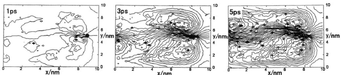
FIG. 2 The time evolution of a STZ with an introduced screw dislocation. The contour lines show the magnitude of the z-displacement after the application of shear stress.
