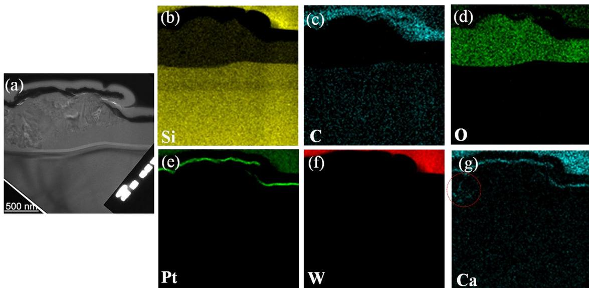
Fig.3 (a) Cross-sectional TEM image and (b)-(g) XEDS elemental maps of Si, C, O, Pt, W and Ca corresponding to Fig.3 (a), respectively.
