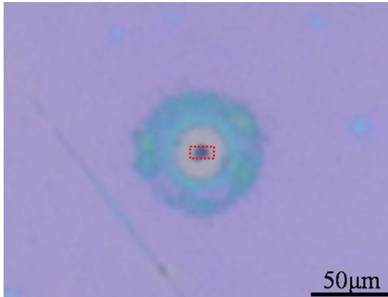
Fig.1 Optical microscope image of the Si-terminated face of the sample after being oxidized at 1473K for 25 hours.
