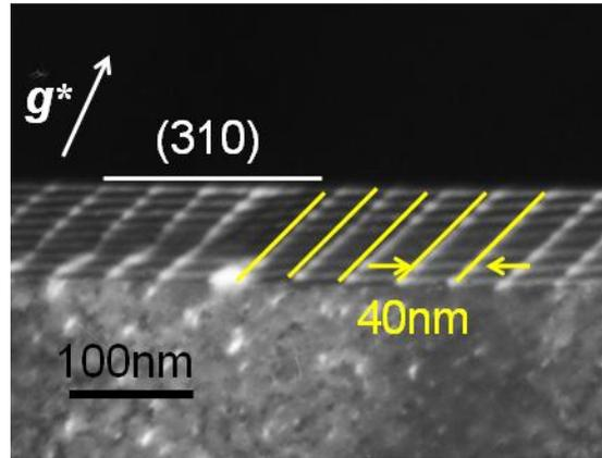
FIG. 1 Dark-field TEM image of MgO bicrystal  $\Sigma 5$  boundary.
