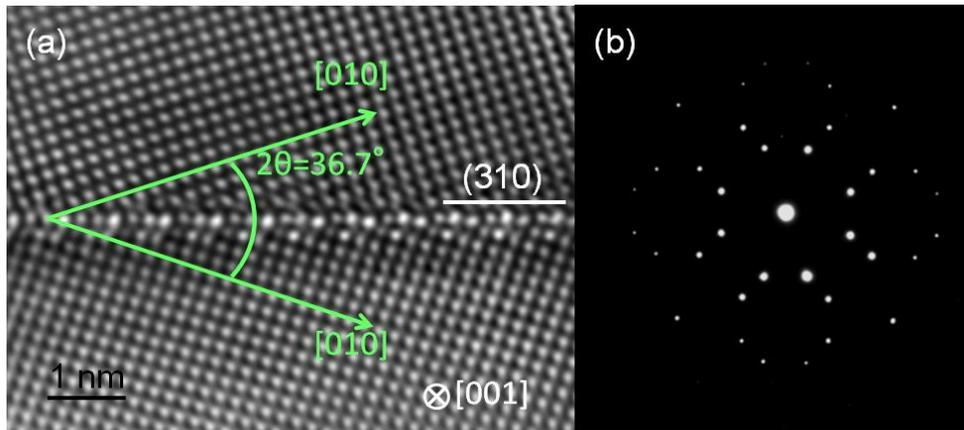
FIG. 2 (a) High-resolution TEM image and (b) selected area diffraction pattern of MgO bicrystal  $\Sigma 5$  boundary.
