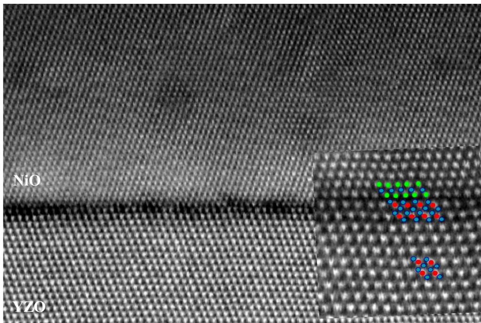
FIG.2 a) HAADF from the NiO(111)/YZO(111). b) HAADF from the near interface region from NiO/YZO showing the abruptness of the interface and its atomic structure. Filled circles represent atomic column of O (blue), Y/Zr (red), and Ni (green).
