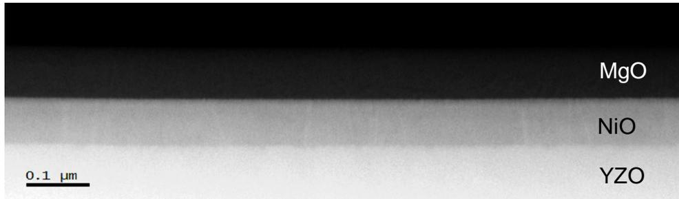
FIG.1. Low magnification HAADF image from MgO/NiO/YZO multilayer film.
