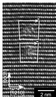
FIG. 3. A HRTEM image of a basal dislocation formed at the boundary in a  $\text{LiNbO}_3$  bicrystal.
