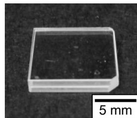
FIG. 1. Optical micrograph of the fabricated  $\text{LiNbO}_3$  bicrystal.
