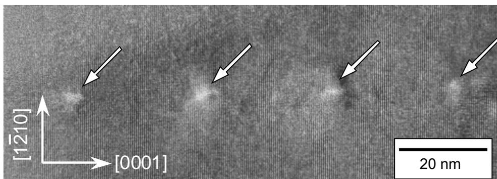
FIG. 2. Boundary dislocation array at a  $\{\bar{1}2\bar{1}0\} / \langle 10\bar{1}0 \rangle$  low-angle tilt grain boundary
