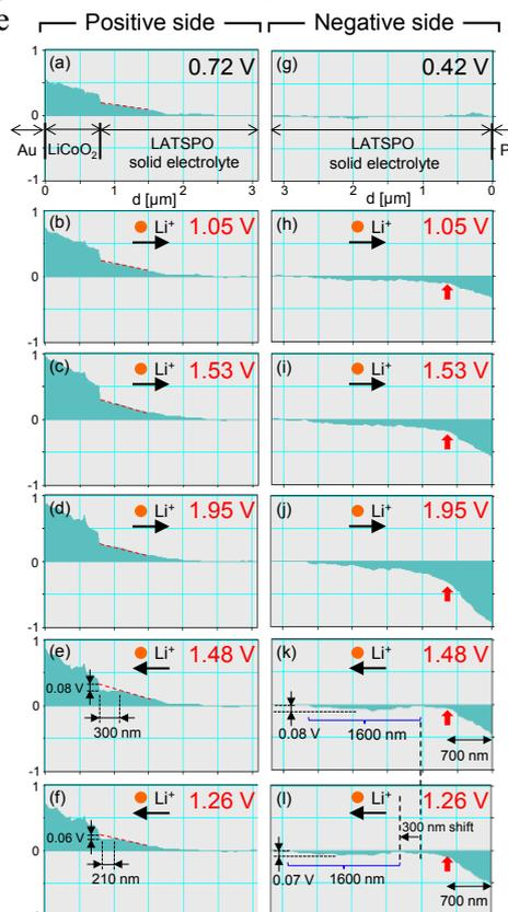
Figure 2 Electric potential profiles obtained from the line "A"- "B" and "C"- "D" indicated in Figs. 1(b) and 1(c), (a) - (f) profiles around the positive side, (g) - (l) profiles around the negative side.
