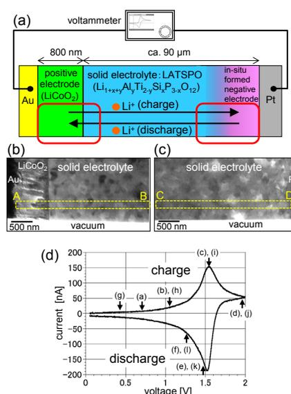
Figure 1 Prepared battery sample, (a) illustration of the battery sample, (b), (c) TEM images around the interfaces, (d) cyclic voltammogram measured in a TEM
