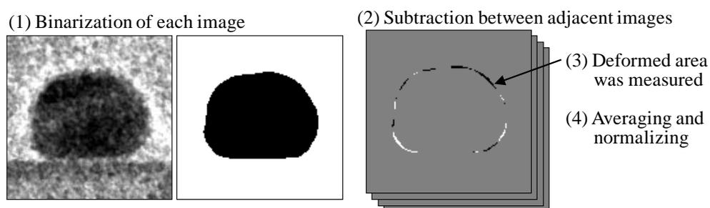
FIG. 1 Evaluation procedures of the deformed values in the series of the ETEM images.
