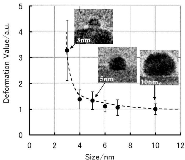
FIG. 2 Size dependency of the deformed value of gold particles, observing under reaction gas condition (1000 Pa; CO + Air).
