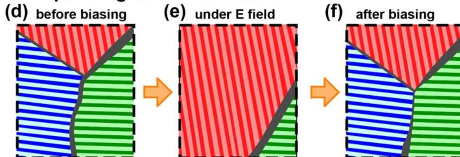
FIG. 2. Dark-field TEM images of PMN-PT single crystals (a) before, (b) during, and (c) after electrical biasing. Schematic of corresponding domain structure (d) before, (e) during, and (f) after electrical biasing.
