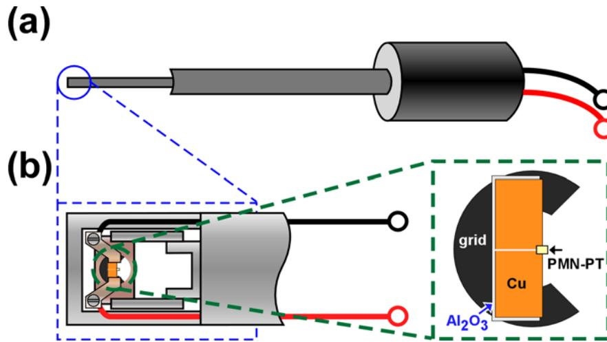
FIG. 1. (a) Schematic of *in-situ* electrical biasing TEM specimen holder (whole view). (b) Magnifications of the holder around the specimen loading part (left) and TEM specimen (right).
