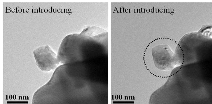
Fig. 2: TEM images of calcium oxide powder before and after high-humidity gas introducing
