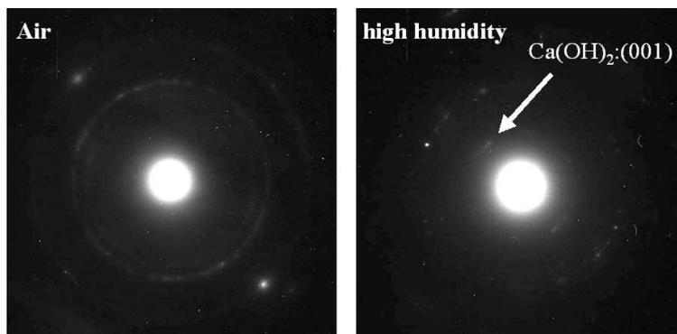
Fig. 1: Electron diffraction patters from samples after air and high-humidity gas introducing
