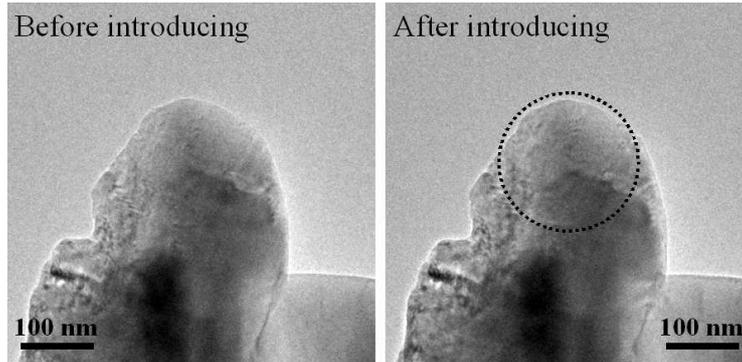
Fig. 1: TEM images of calcium oxide powder before and after Air introducing
