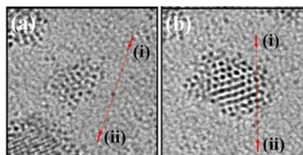
Fig. 3. AC-TEM images of Pt nanoparticles.
