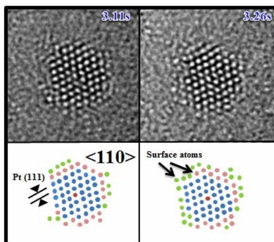
Fig. 5: SAC image of a Pt nanoparticle obtained 3.11 and 3.26s after the start of EM observation.
