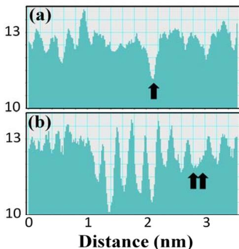
Fig.4 Intensity line profiles corresponding to the 3.5nm distances shown in Fig. 1(a) and (b), extracted using the Digital Micrograph software.
