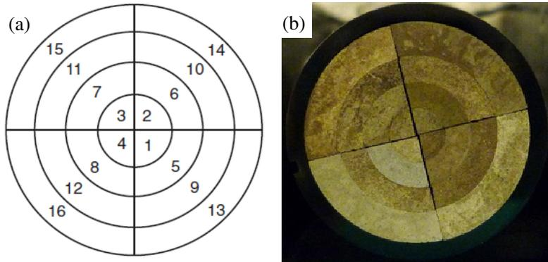
FIG. 1. (a) Schematic and (b) photograph of the new detector showing the 16 individually addressable segments.
