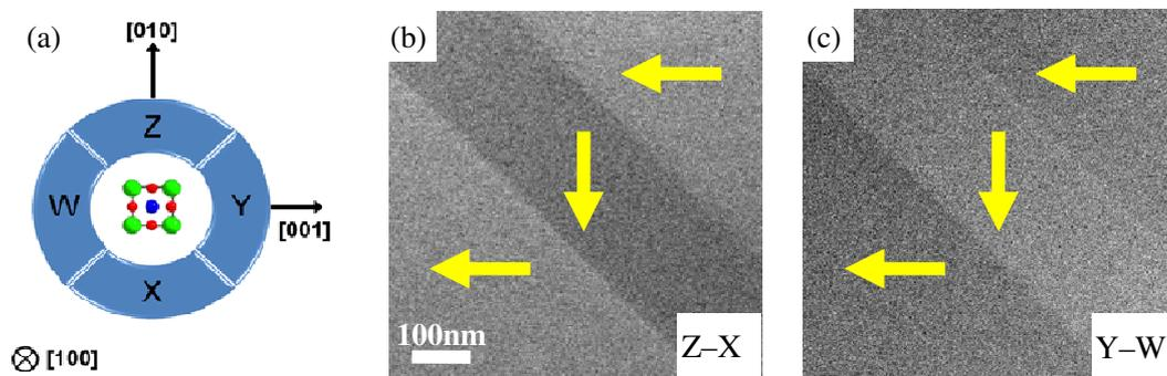
FIG. 3. For the detector orientation relative to  $\text{BaTiO}_3$  crystal shown in (a) (ring 2 only shown), experimental low magnification differential phase contrast images are shown in (b) and (c). The domain structure is clear. Yellow arrows mark the polarization directions.
