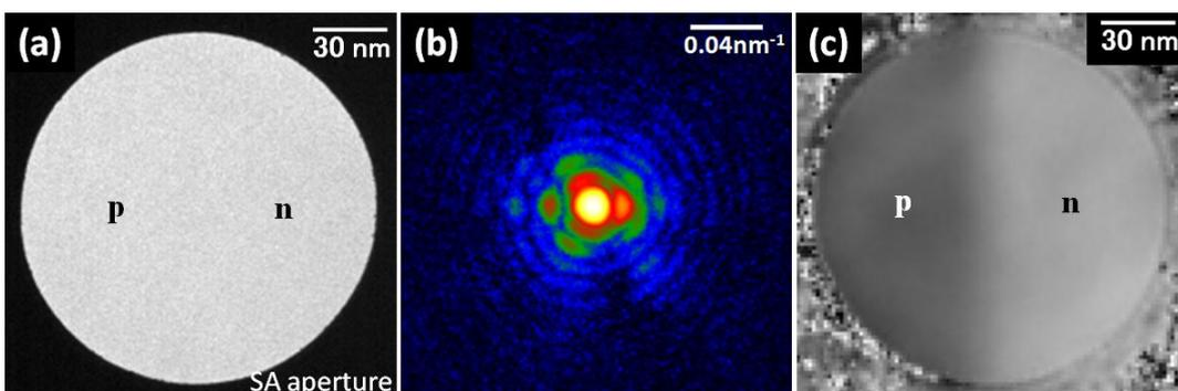
FIG. 3. Reconstruction of the phase image of a p-n junction in GaAs.
