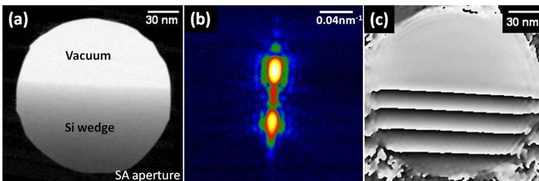
FIG. 2. Reconstruction of the phase image of a wedge-shaped Si crystal.
