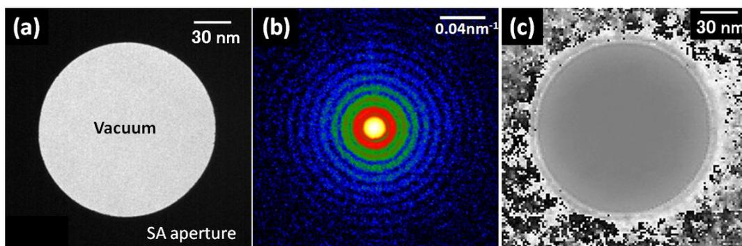
FIG. 1. Phase reconstruction of illumination electron wave by electron diffractive imaging. (a) Bright field TEM image of a selected-area aperture and (b) the corresponding direct spot. (c) Phase reconstructed in the aperture hole.
