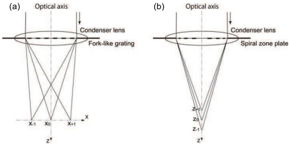
FIG. 2. Schematic raypath diagrams of diffracted waves produced by a fork-like grating (a) and spiral zone plate (b).
