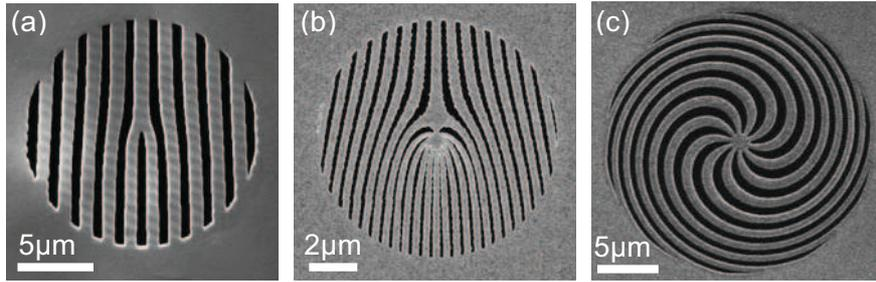
FIG. 1. SIM images of the masks fabricated by an focused-ion-beam instrument. Fork-like gratings with topological charges of 1 (a) and 10 (b), and a spiral zone-plate with a topological charge of 10 (c).
