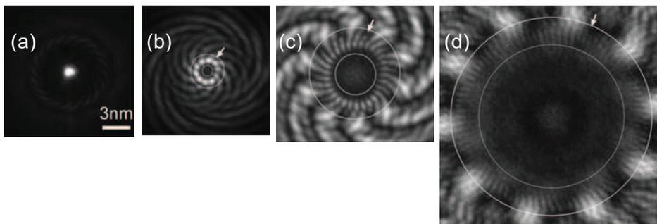
FIG. 4. A series of vortex waves focused at different  $z$ -positions, which are produced by the fork-like grating shown in FIG.1(b).
