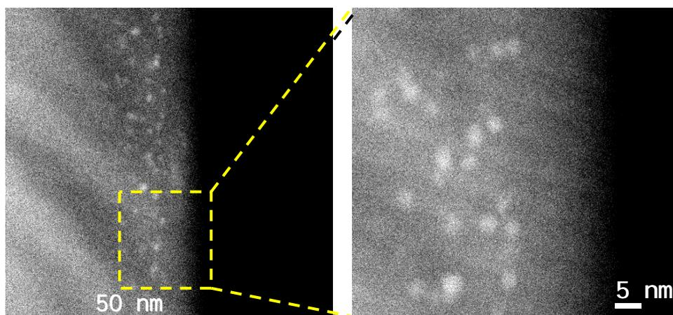
FIG. 2 HAADF-STEM images of the sample implanted at the fluence of  $2 \times 10^{15} \text{ cm}^{-2}$ , irradiated with X-ray and exposed to the air, taken by Jeol ARM200F operated at 80 kV.
