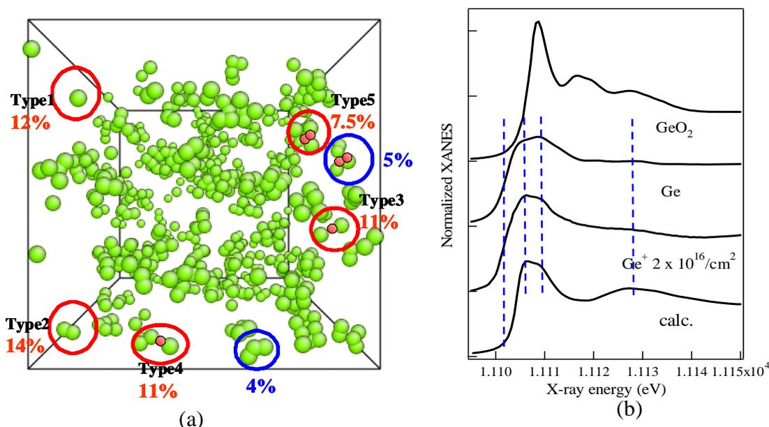
FIG. 1 (a) Perspective view of spatial distribution of Ge atoms in silica glass, derived by RMC fit to EXAFS of the sample implanted at the fluence of  $2 \times 10^{16} \text{ cm}^{-2}$ . (b) Experimental Ge K-edge XANES of pure Ge,  $\text{GeO}_2$ , the implanted sample and theoretically calculated XANES by FEFF code, based on the model obtained by RMC-EXAFS fit (a).
