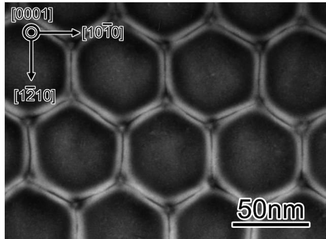
FIG. 2. A bright-field TEM image of the grain boundary observed in plan-view. A hexagonal screw dislocation network is formed.
