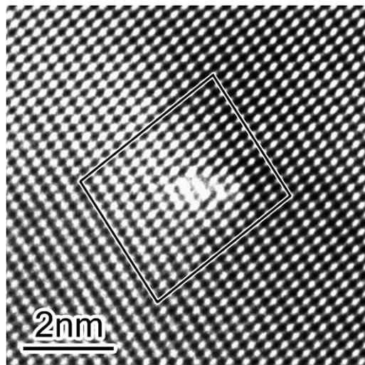
FIG. 3. A high-resolution TEM image of a screw dislocation core observed end-on. The screw dislocation is not dissociated.
