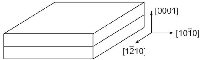
FIG. 1. A schematic illustration showing the bicrystal fabricated in this study. The bicrystal contains a (0001)/[0001] low-angle twist boundary.
