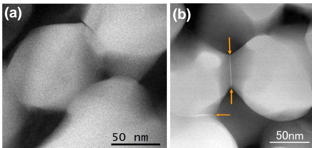
**Fig.2** HAADF-STEM images of 0.1 mol% Y<sub>2</sub>O<sub>3</sub>-doped Al<sub>2</sub>O<sub>3</sub> sintered at (a) 1100°C, and (b) 1200°C. In (b), the arrows are showing line contrasts.
