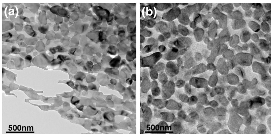
**Fig.1** TEM bright field images 0.1 mol% Y<sub>2</sub>O<sub>3</sub>-doped Al<sub>2</sub>O<sub>3</sub> sintered at (a) 1100°C, and (b) 1200°C.
