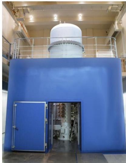
FIG. 3. 1.2-MV field-emission holography electron microscope.
