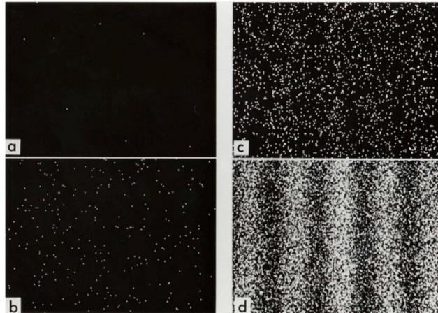
FIG. 1. Build-up of an electron interference pattern.
