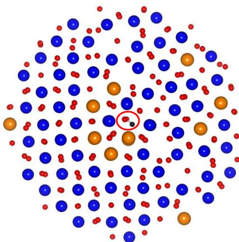
Fig. 2: Schematic of the lowest energy configuration for a proton-doped 14 mol% YSZ  $\Sigma 5(310)/[001]$  grain boundary.
