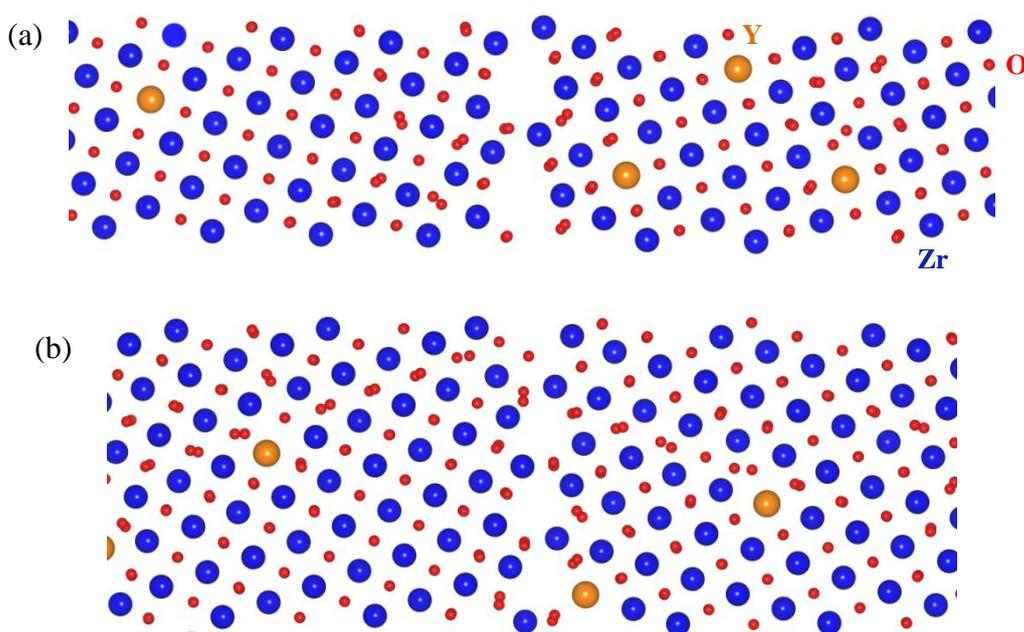
Fig. 1: Example configurations for the (a)  $\Sigma 5(210)/[001]$  and (b)  $\Sigma 5(310)/[001]$  grain boundaries in 3.5 mol% YSZ.
