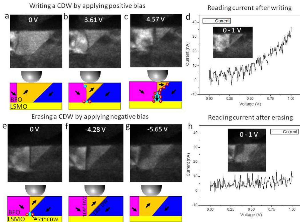
FIG. 2. (a)-(c) Dark-field diffraction contrast TEM images extracted from a video showing writing a CDW by applying a positive bias ramp. (d) Current measured by applying a low reading voltage after writing. (e)-(g) Dark-field diffraction contrast TEM images extracted from a video showing erasing a CDW by applying a negative bias ramp. (d) Current measured by applying a low reading voltage after erasing.
