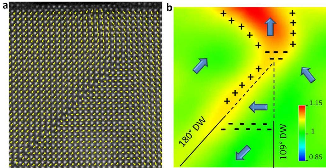
FIG. 1. (a) Plot of the  $-\mathbf{D}_{\text{FB}}$  vectors overlaid on HAADF image of a  $109^\circ/180^\circ$  domain wall junction near the free surface of the 20 nm thick  $\text{BiFeO}_3$  film. (b) The corresponding color map of the  $c/a$  ratios. The polarization orientation and bound charge are indicated schematically.
