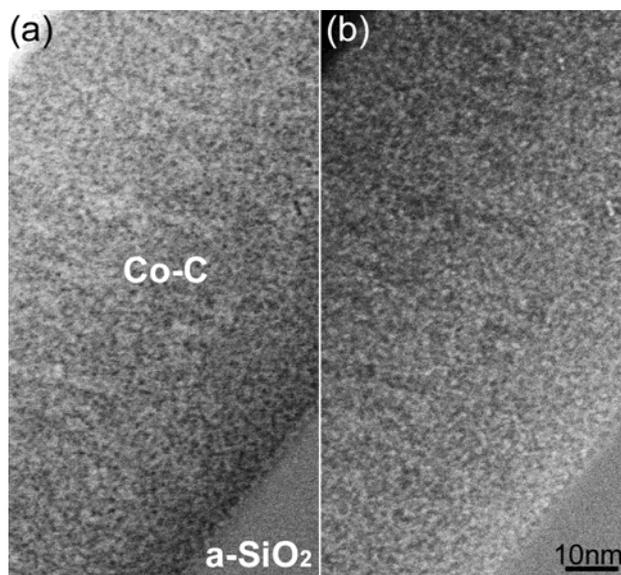
FIG. 1. A pair of (a) BF-STEM and (b) HAADF-STEM images of a cross section of the Co-C granular thin film. For the HAADF-STEM imaging, a beam convergence of 10 mrad and a detector inner angle of 60 mrad were used.
