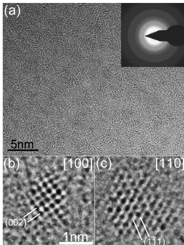
FIG. 2. (a) Cs-corrected HRTEM image and the corresponding SAED pattern of the cross section of
