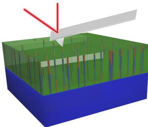
**Fig. 1** A schematic of atomic scale ferromagnetic dislocations embedded in antiferromagnetic NiO. The blue block is SrTiO<sub>3</sub> substrate and the green block is NiO single crystalline thin film. The red/blue cylinders are magnetic dislocations in NiO film. The AFM and MFM observations are carried out on the surface of film.
