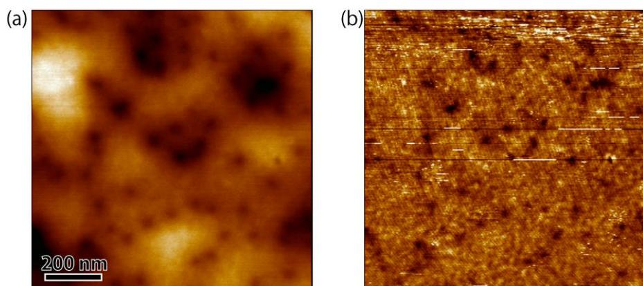
**Fig. 2** (a) AFM topographic image and (b) MFM phase image of the NiO thin film. Dark spots in AFM topographic image correspond to the dislocations. MFM image was taken 20 nm above the surface to reduce the effect of atomic force.
