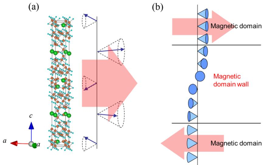
FIG. 2. (a) Crystal and magnetic structures of  $\text{Sr}_3\text{Co}_2\text{Fe}_{24}\text{O}_{41}$ . The small and large arrows represent the magnetic moments for the respective layers and the unit cell, respectively. (b) A possible model of the magnetic domain wall structure in  $\text{Sr}_3\text{Co}_2\text{Fe}_{24}\text{O}_{41}$ .
