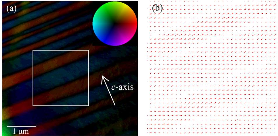
FIG. 1. (a) Magnetization-distribution map of  $\text{Sr}_3\text{Co}_2\text{Fe}_{24}\text{O}_{41}$  derived by the transport-of-intensity equation (TIE) method. The inset is a color wheel for interpretation of the color distribution map. (b) Local magnetization distribution from TIE for the boxed region in (a).
