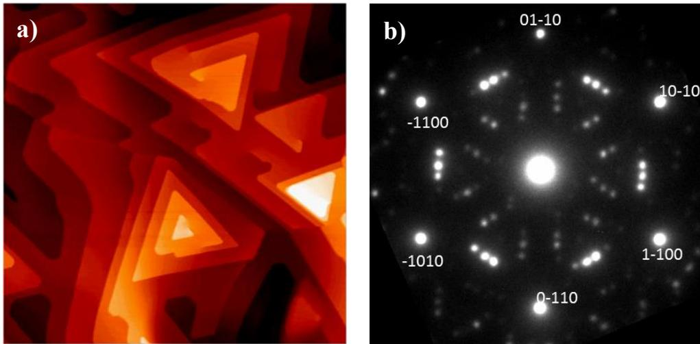
FIG. 1. a) STM image from the spiral growth of  $\text{Bi}_2\text{Se}_3$ . B) plan view selected area diffraction of region showing the epitaxy between the SiC substrate and the  $\text{Bi}_2\text{Se}_3$  film. The substrate SiC(0001) diffraction spots are indexed.
