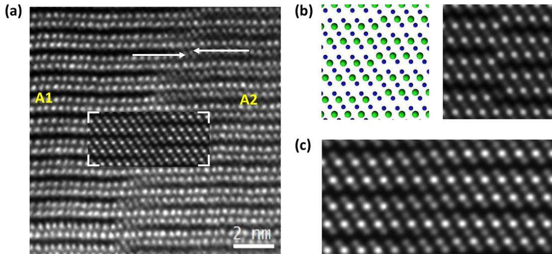
FIG. 2 a) Cross-sectional HAADF image from a region that contain antiphase domain boundary. b) Atomic model of the edge on antiphase boundary and corresponding calculated HAADF map. c) HAADF calculated map for tilt boundary of five degree.
