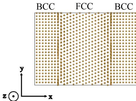
Fig. 1 An example supercell of  $\delta/\gamma$  interface and optimized atomic configuration. Distortion of bond was confined within 5 Å at either side of the interface.
