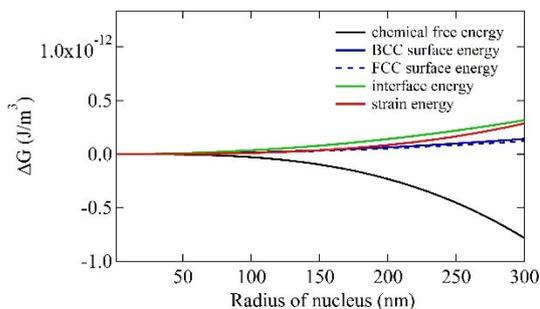
Fig. 3 Free energy change upon nucleation as a function of radius of nucleus at  $\Delta T = 100$  K.
