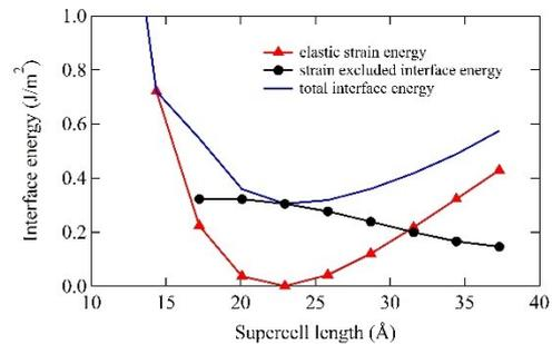
Fig. 2 Strain-excluded interface energy as a function of supercell length along  $z$ -axis, in comparison with cell strain energy in 10 Å wide interface region.
