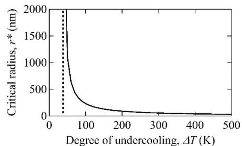
Fig. 4. Critical radius as a function of undercooling. Dashed line at  $\Delta T \sim 30$  K indicate threshold for nucleation.
