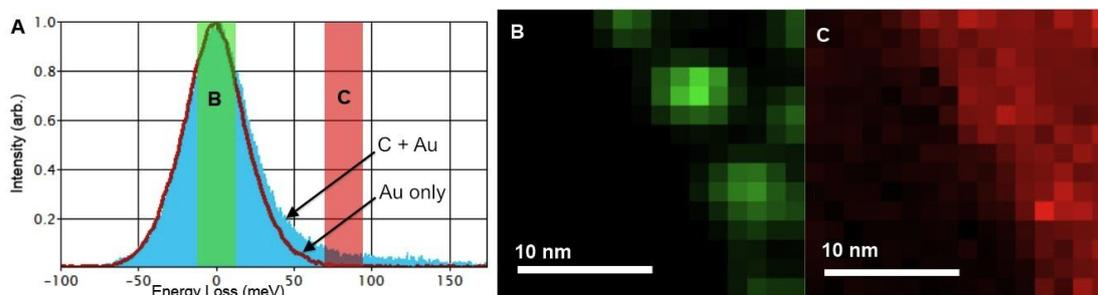
FIG. 3. Energy-filtered HAADF imaging of Au particles on amorphous carbon. A (line): spectrum from Au particles; A (solid) spectrum from carbon plus Au; B: image formed with an energy window of  $0 \pm 10$  meV; C: image formed with an energy window of  $85 \pm 10$  meV.
