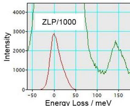
FIG. 2. Optical phonon in  $\text{SiO}_2$ . ZLP tail is reduced to 1/3000 at 100 meV.
