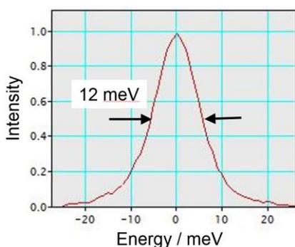
FIG. 1. EELS Zero Loss Peak (ZLP) recorded by HERMES in 0.25 sec.  $E_0 = 60$  keV.
