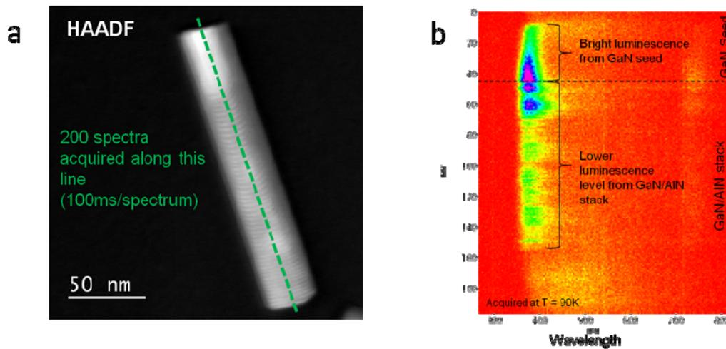
Fig. 2. CL-SI study of a nanorod of GaN/AlN heterostructure
