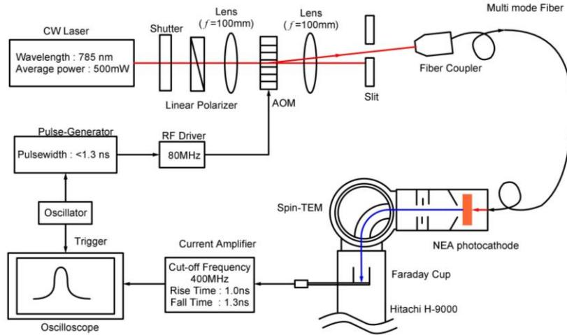
FIG. 1. Schematic diagram of a measurement system for the time structure of pulse beam by using a Faraday-cup current monitor in SP-TEM.
