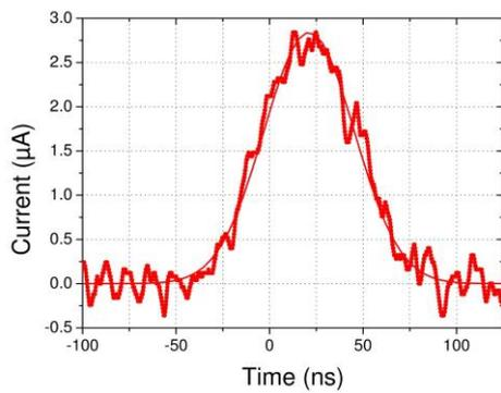
FIG. 3. A time structure of pulsed electron beam.
