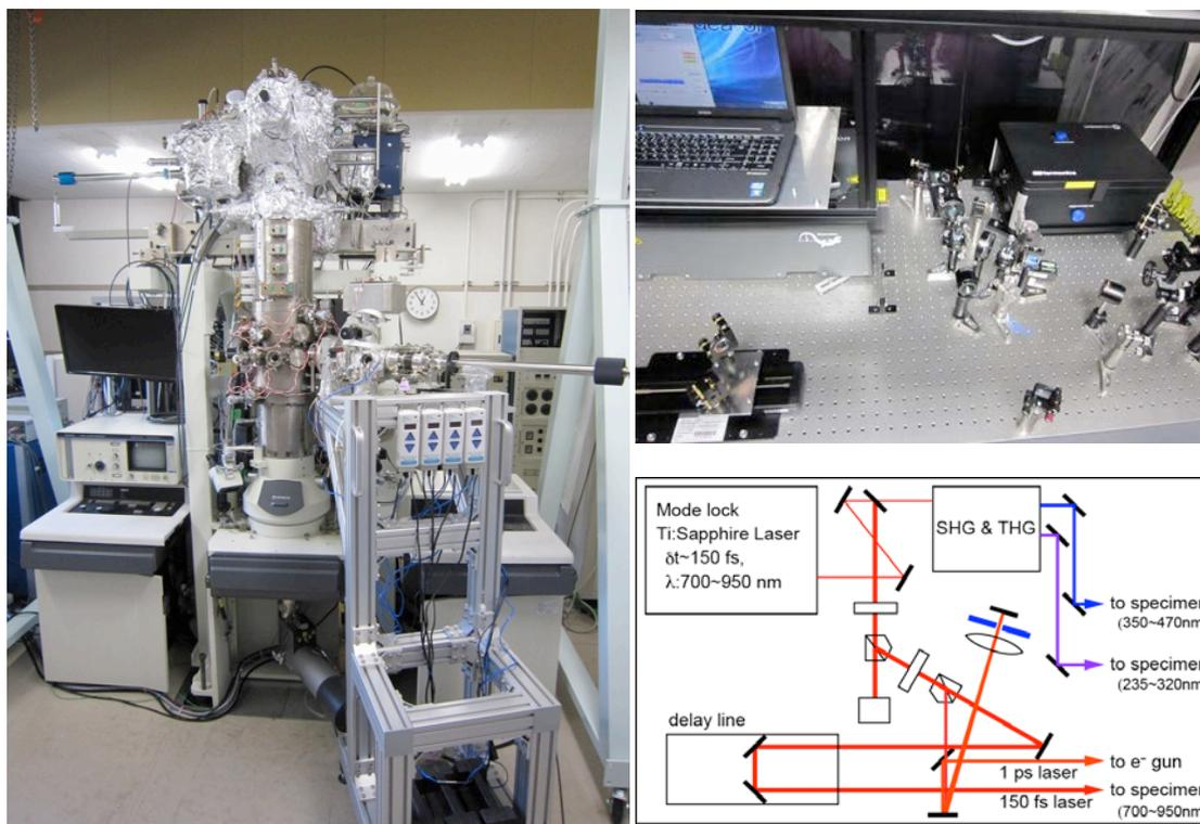
FIG. 1. Photograph of the SP-TEM and the optical system on optical bench. (Left) elevation view of the SP-TEM, (Upper right) femto second pulse laser system for pulse-mode operation for pump-probe measurement in SP-TEM. (Right bottom) schematic diagram of the pulse laser system.
