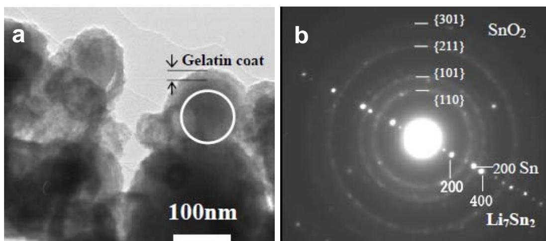
FIG. 2 (a) TEM image of lithium charged gelatin-coated Sn particles. The gelatin coating is retained after lithiation. (b) The electron diffraction pattern obtained from the white circle in (a). Li<sub>7</sub>Sn<sub>2</sub> phase is indexed as well as Sn and SnO<sub>2</sub>.
