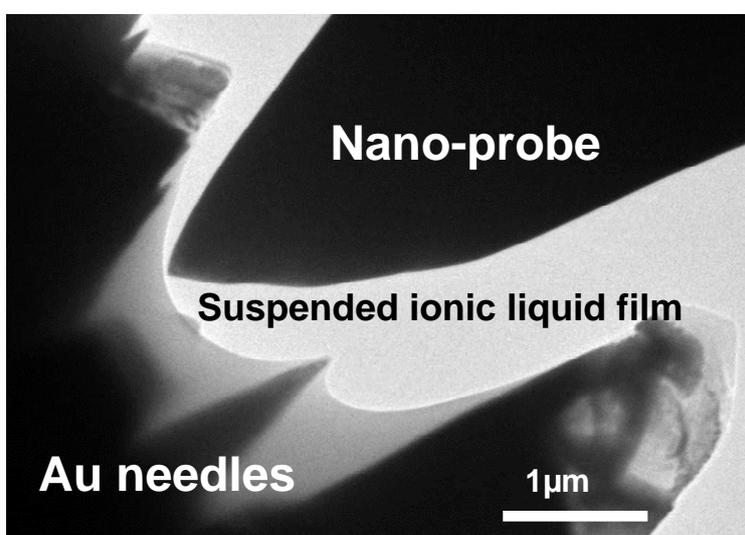
FIG. 1. An agar-based ionic liquid film suspended between gold needles
